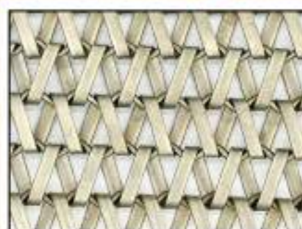
Material: SS201, 302, 304, 316 Cross/Spiral diameter: 2.0mm/1*4mm Cross/Spiral pitch: 15mm/10mm
