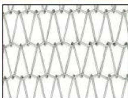
Material: SS201, 302, 304, 316 Cross/Spiral diameter: 1.5mm/1.2mm Cross/Spiral pitch: 16mm/6mm
