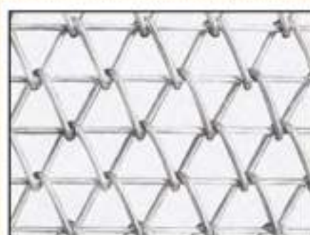
Material: SS201, 302, 304, 316 Cross/Spiral diameter: 1.5mm/1.5mm Cross/Spiral pitch: 13mm/11mm
